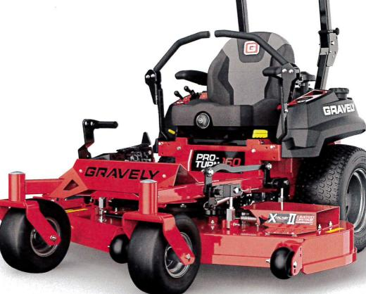
X-FACTOR® II DECK The 7-gauge, all-steel welded X-Factor® II Deck is fabricated from top to bottom, providing industrial-strength peace of mind that's reinforced with an exclusive limited lifetime warranty.
