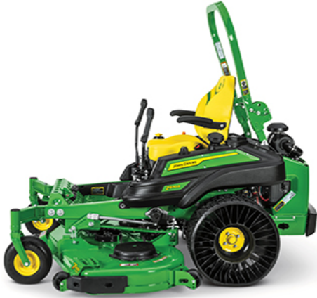
Z970R shown with optional X® Tweel® Turf airless radial tire technology
